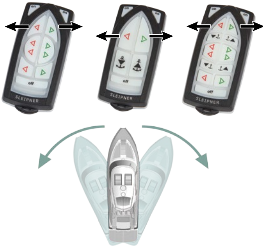
Activating the bow thruster
