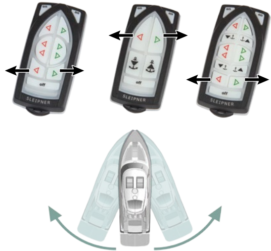
Activating the stern thruster
